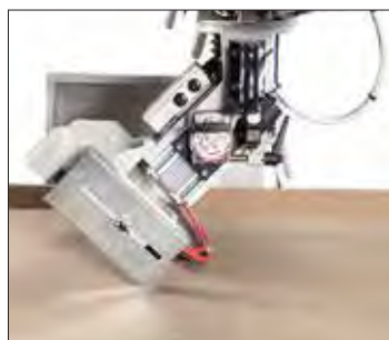
Vertical pneumatic clamp.
